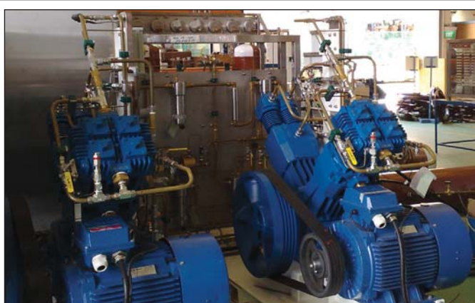
Hycomp Heliox compressors being tested within the LexMar's LESGAZ Diver Gas Reclaim System at their Singapore location.
